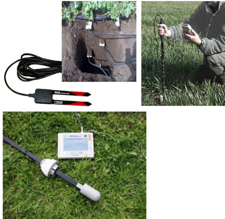
Figure 14 Some examples of field sensors for moisture monitoring. From left to right: Decagon ECH2O series sensors (placed at different depths); DeltaT PR2 probe; Sentek Diviner probe
