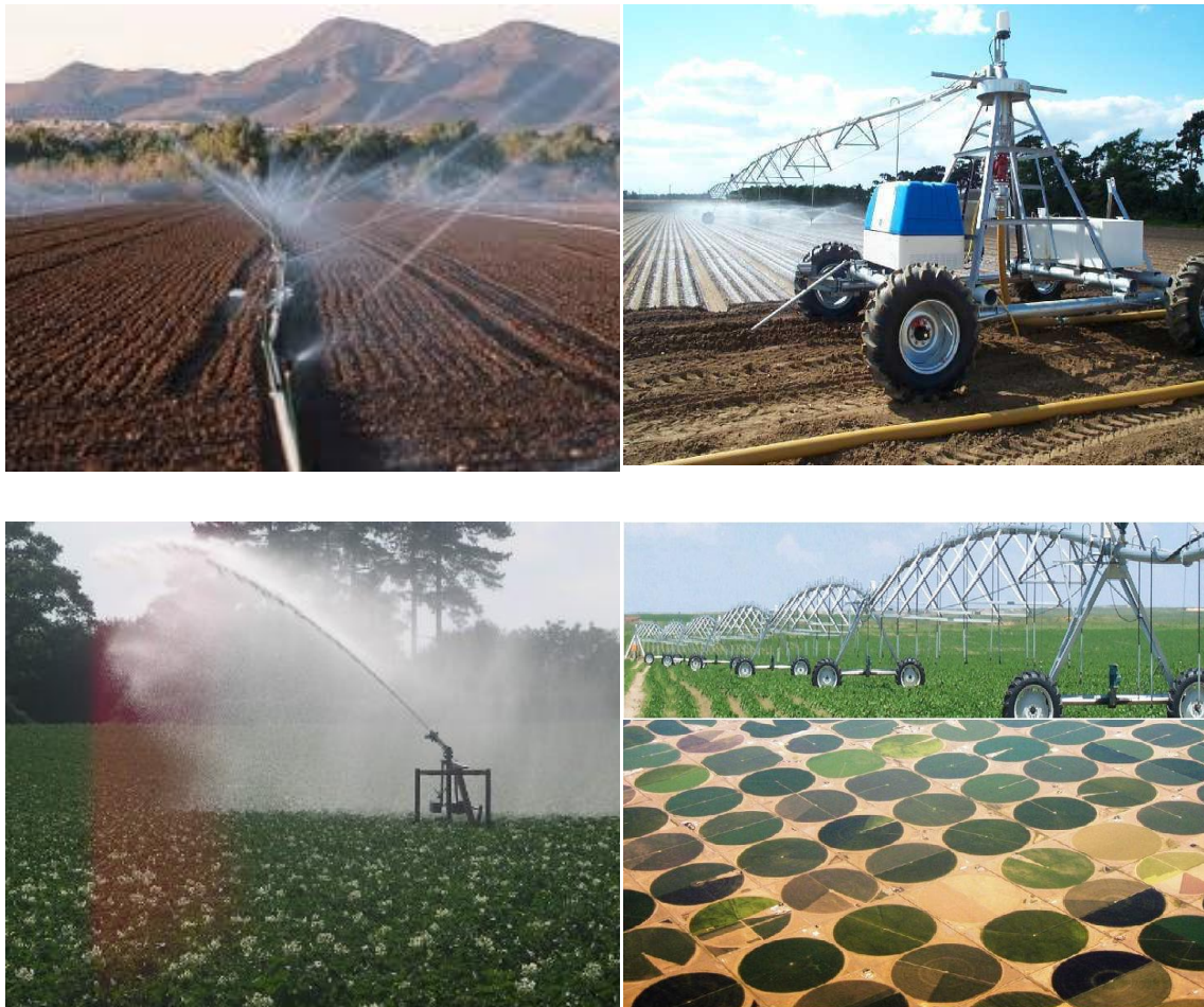
Figure 20 Examples of sprinkler irrigation systems (from top-left to bottom-right): rotary set-sprinklers; moving laterals; moving guns; center pivot.
